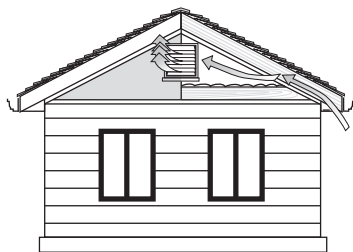
The gable-louver vent, an exhaust vent, allows unwanted air to flow out of the attic.
