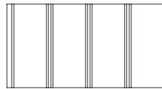
TRULINE® HP & TS 16" Soffit - Solid HP: 16SS TS: 16SS_BLDR Aluminum 0.019" & 0.016"
